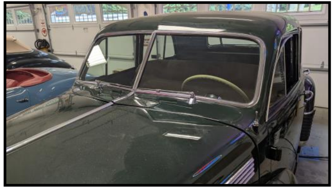
The restored vacuum antenna and wipers installed
