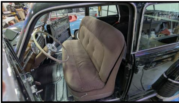
The front seat has been installed so that road testing can begin before it gets cold
