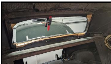
Wood Panel Bonded To Car
