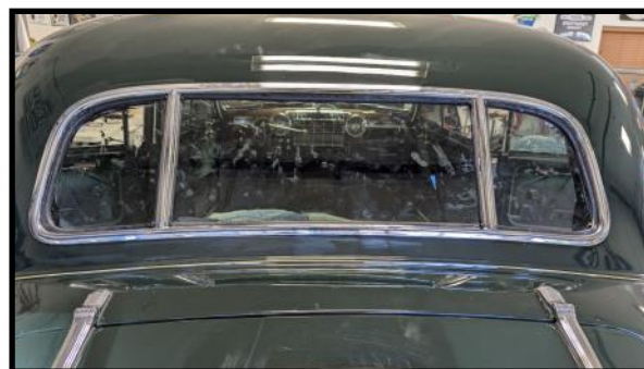
Rear Window Frame & Glass Installed
