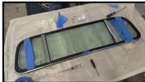
Dry Fitting Rubber Rear Glass & Trim
